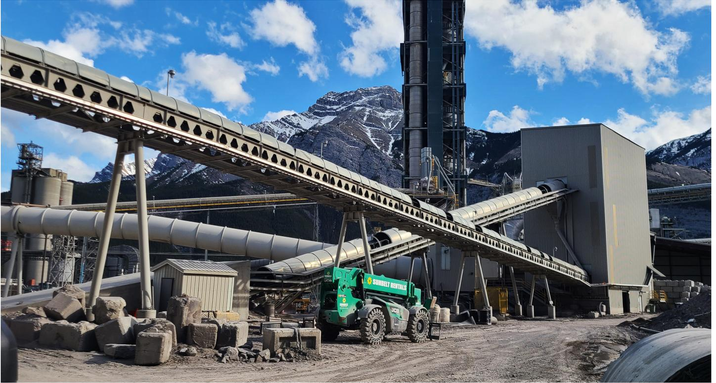
In your operations, you handle a significant volume of rugged materials like ore, aggregates, crushed stone, solid rocks, sand, and gravel. Your conveyor belting must not only be reliable and consistently efficient, but also tough enough to endure the severe operating conditions. These extreme conditions can cause your belting to suffer gouges, tears, rips, and abrasion, leading to premature failures, operational downtime, and increased maintenance costs.
