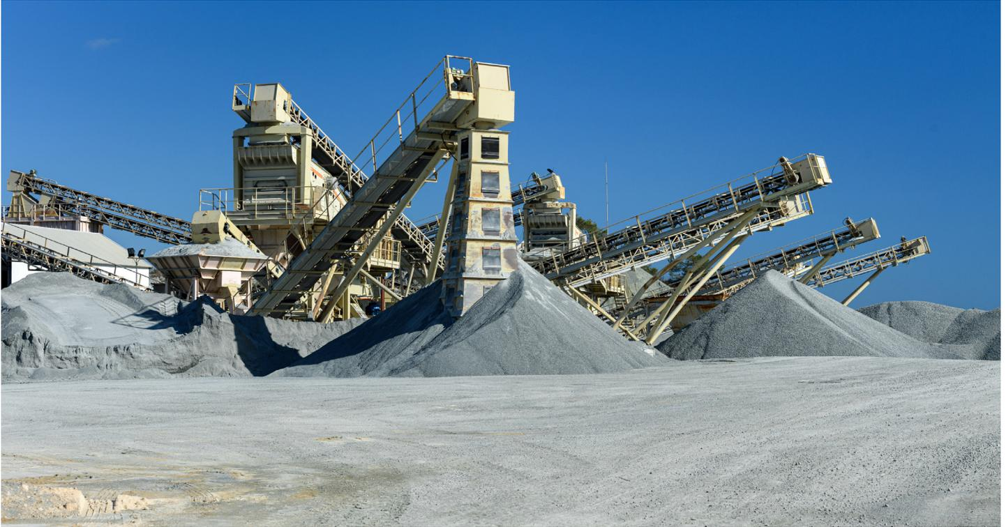
Extreme hard-rock mining subjects belts to constant severe abrasion which can cut short your belt's lifespan.
